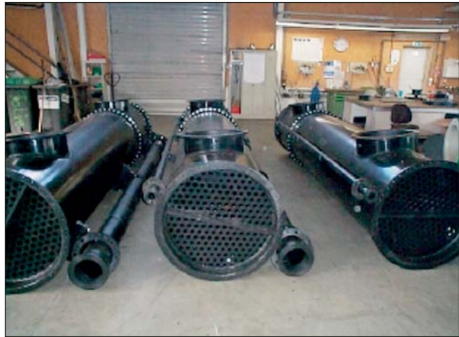
Stripper towers are used for the treatment. The process has to be operated with a specific water-air ratio due to the water solubility of MTBE.
