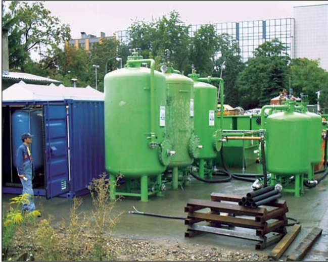
The treatment plant with a pre-settling stage, a filter stage, a liquid phase activated carbon stage, as well as ion exchangers for the removal of cyanides.
