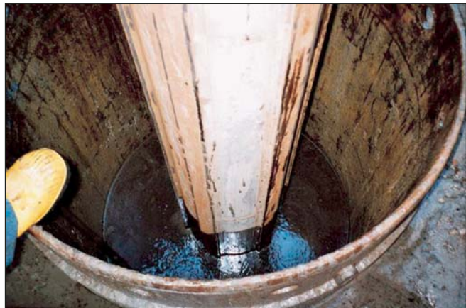
Free tar phase was monitored in the boreholes several times on top of the groundwater.
