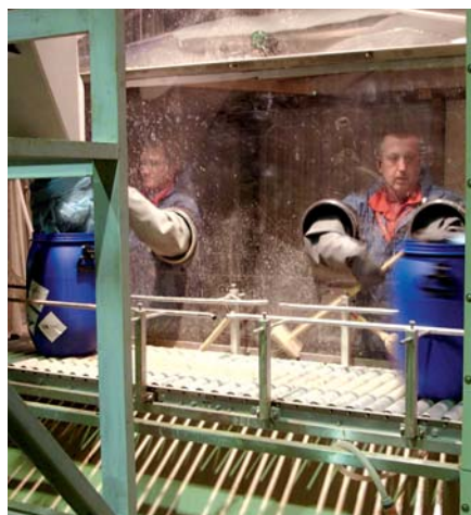
▲ Handling of the barrels using a specially developed glove box
